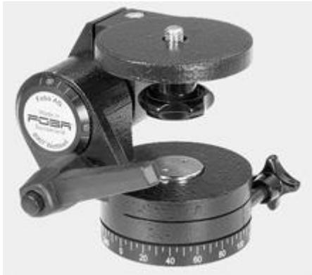
Tilting head with one tilt axis through over 90°. Fixation with locking lever (Quick-Lock). The tilt axis has a graduation ranging from -15° to +105°, labelled in intervals of 15°; incl. 3/8" camera screw (1/4" available upon request). The camera plate is provided with a round level.
