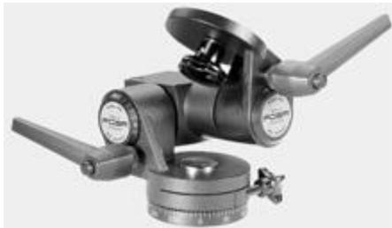
Dual tilting head with two tilt axes through over 90°. Fixation with locking lever (Quick-Lock). The tilt axes have a graduation ranging from -15° to +105°, labelled in intervals of 15°; incl. 3/8" camera screw (1/4" available upon request). The camera plate is provided with a round level.
